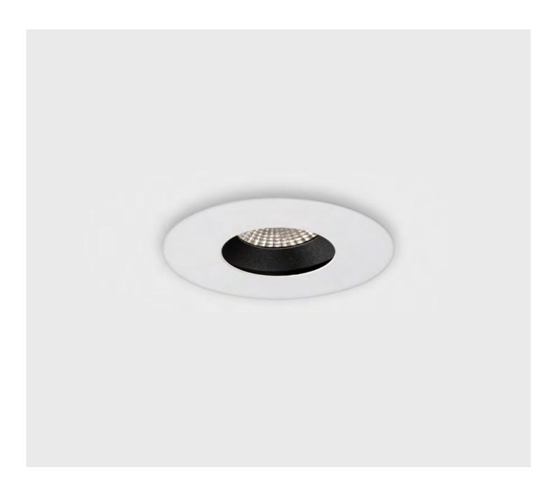
Lila is a range of recessed luminaires dimmable LED modules with up to 1100lm lumen output. Available with a round pinhole or oval keyhole aperture, Lila achieves high-intensity, accent lighting with no light spill. Both versions can be tilted up to  $\pm 25$  degrees and the downlight has a black internal surface and is deep set for glare control and optimal visual comfort. Lila downlights are suitable for use in residential, retail and various other indoor applications.
